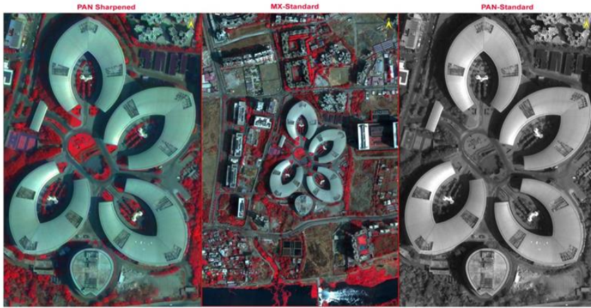
AOI: EON IT Park ,Pune Cartosat-3 45cm PAN Sharpened, 1.1m MX and 45cm PAN
