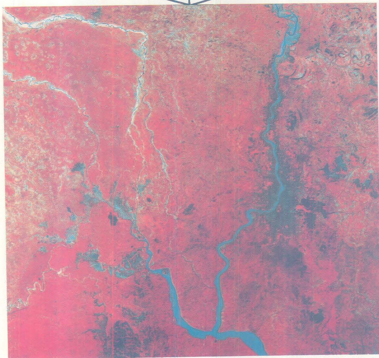
Figure 2.3.2.2 IRS-1D LISS-III FCC image (bands 2,3,4) and corresponding black and white images of band 2, band 3 and band 4 data of path 108, row 56 showing Calcutta and surrounding areas.
