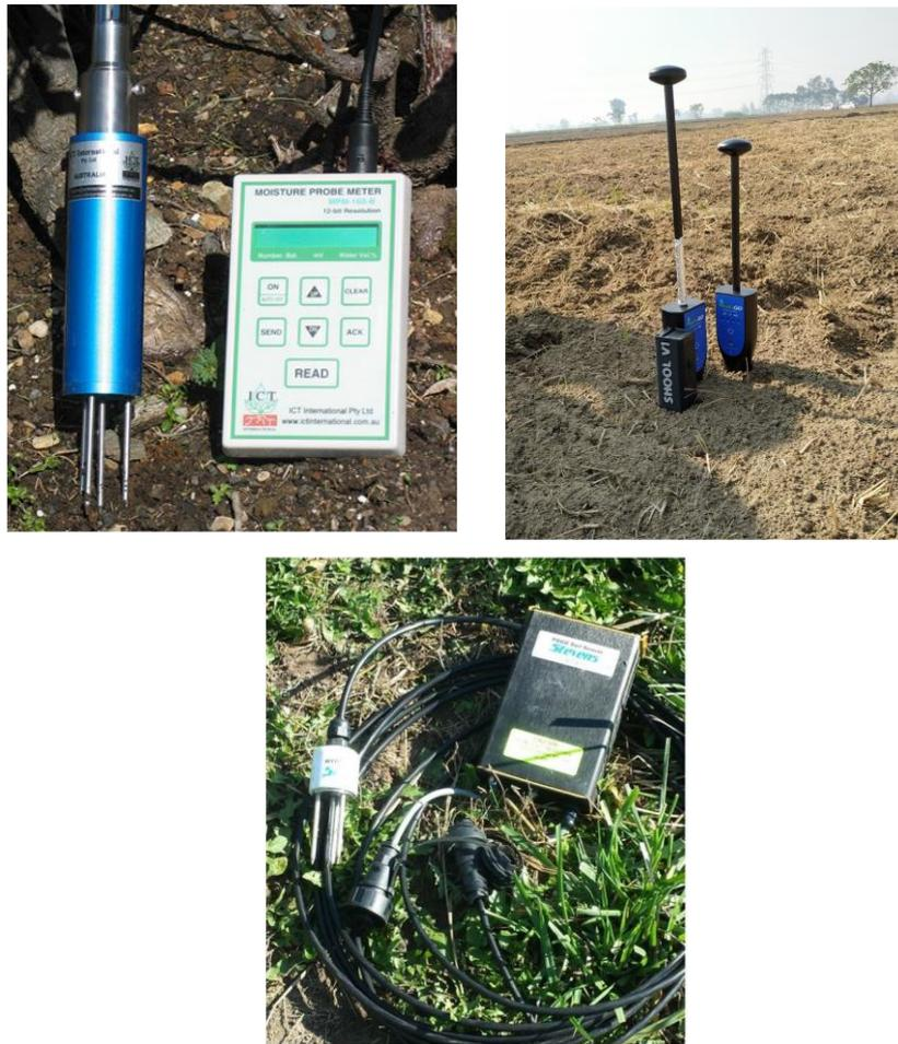
Figure 7: Soil moisture probes for field measurements
