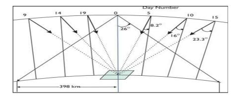
Figure 8.30 Steerability of LISS-IV camera
