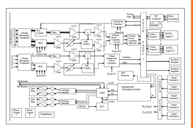
Fig. 5.6 Block Schematic of Data Receive system
