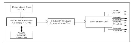
Fig. 5.14 Functional Block diagram of data serializer system
