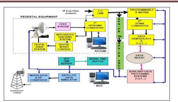
Fig. 5.5 Data Reception System Block
