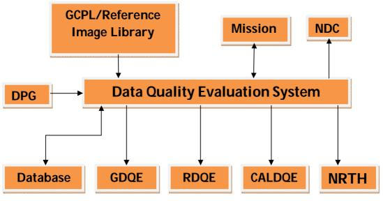
Fig. 7.1 Block Diagram of Data Quality Evaluation System
