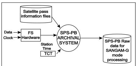
Fig. 5.9 Context diagram of SPS-PB data
