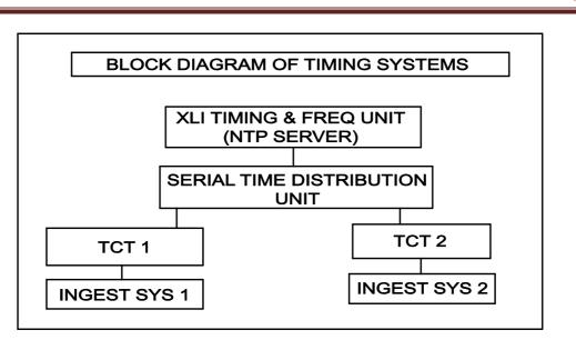
Fig. 5.12 Block diagram of Timing Systems
