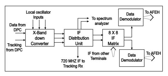
Figure 5.1 Block Diagram of IF and Base Band Systems
