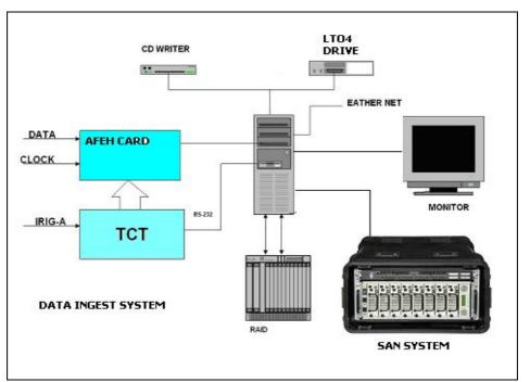
Fig. 5.8 Direct Ingest System
