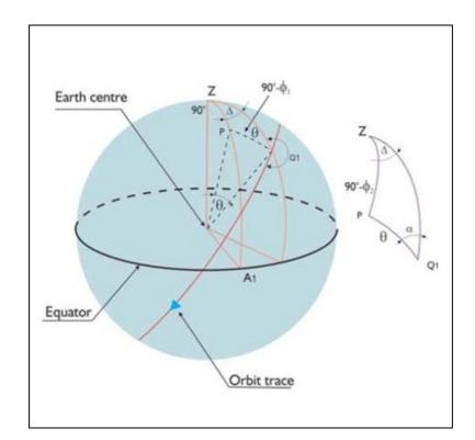
Figure 3.9 Calculations of coordinates of a point P on the earth surface.
