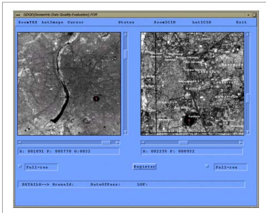
Screen layout for GCP Id when reference is LISS-III / PAN image with rectified corner coordinates
